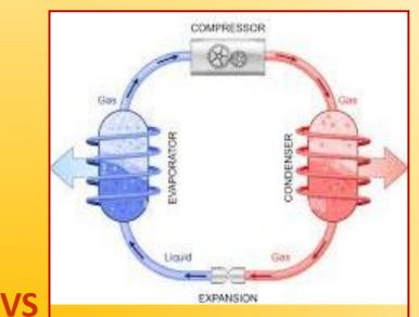
Heat Pumps use a 'heat exchanger' to remove heat from the external environment and to use that heat for hot water and central heating. They use some electricity to run, but convert roughly 3-4 times this amount of energy into heating, so are ultra efficient, and can replace gas boilers entirely.
